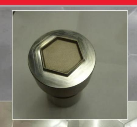
30mm diagonal hex shape in 1.5mm stainless steel (Tool etch# 04147062)
