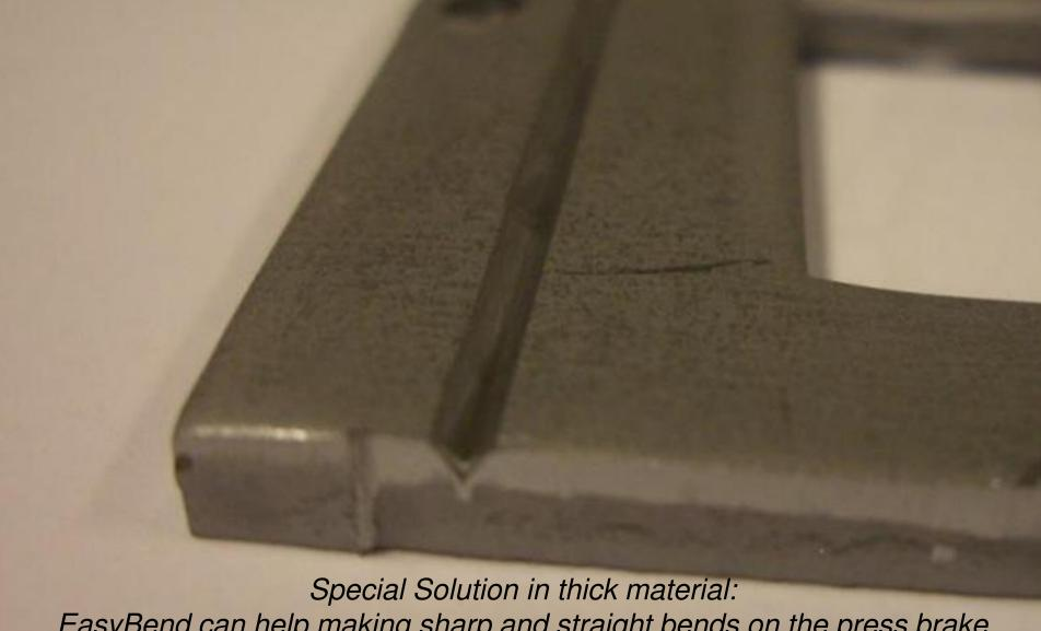
EasyBend can help making sharp and straight bends on the press brake
