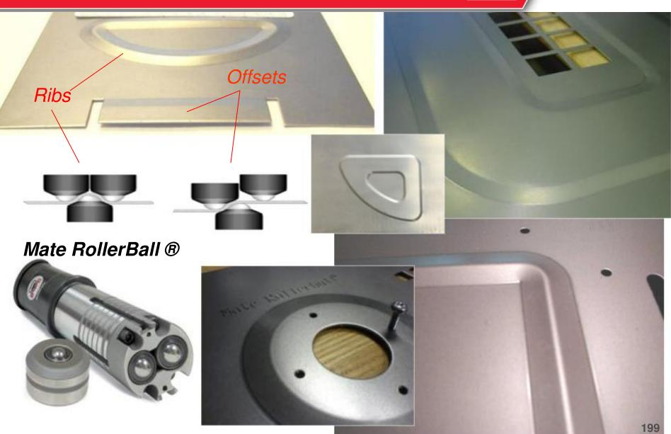
Note: Machine must be able to work in Ram Down mode.
